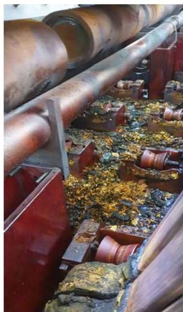
Figure 20. Residues resulting from the chromium plating technological process
