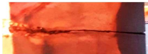
Figure 18. Copper bar breakage due to fatigue corrosion
