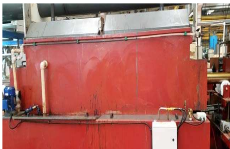
Figure 2. Electrolytic tank in which chromium plating takes place
