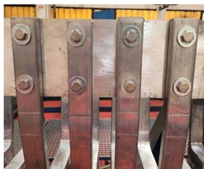
Figure 5. How to attach the anodes to the electrolytic copper bar
