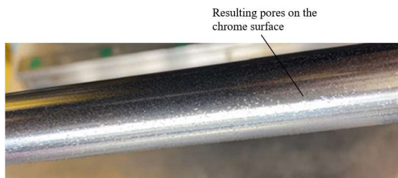
Figure 19. Defects in chrome plating bars
