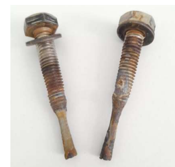
Figure 17. Corrosion of clamping bolts
