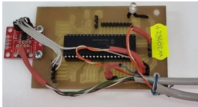
Fig. 3 – Sparkfun development board and RS485 communication module.
