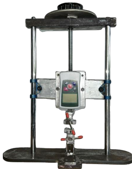
Fig. 5 – Experimental Setup of the Mini-Tensile Tester.
