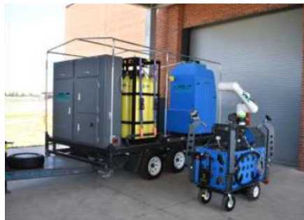
Fig. 1 – Cold Spray installation, VRC Raptor model ( https://vrcmetalsystems.com/ ).
