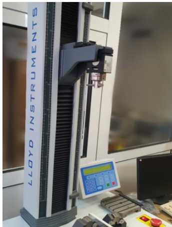
Fig. 9 – Traction test equipment Lloyd Instruments.
