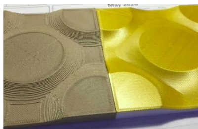
Fig. 3 – Comparison between surfaces obtained by conventional 3D printing.
