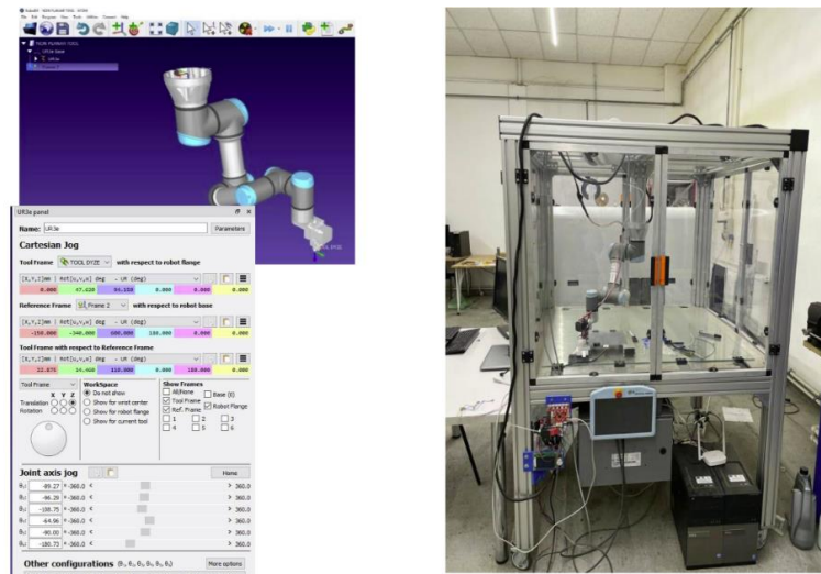
Fig. 5 – Virtual robotic workstation development in RoboDK vs. real workstation.
