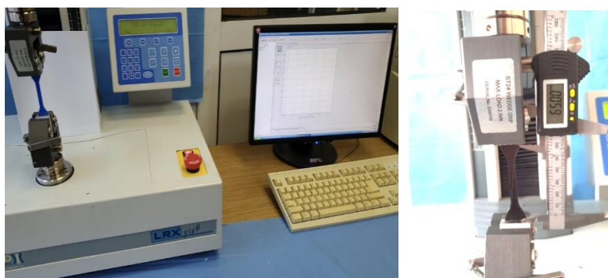
Fig. 11 – Traction test carried out on Lloyd Instruments.
