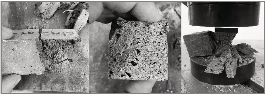
Fig. 1 The determination of compressive strength (testing at 0.5kN/s)
