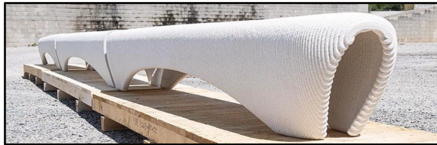
Fig. 4 A 3D printed collection of outdoor furniture made with concrete by the designer Philipp Aduatz
