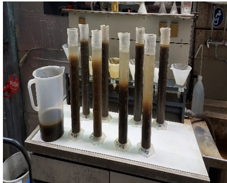
Fig. 5 – The 30 minutes sedimentation test.
