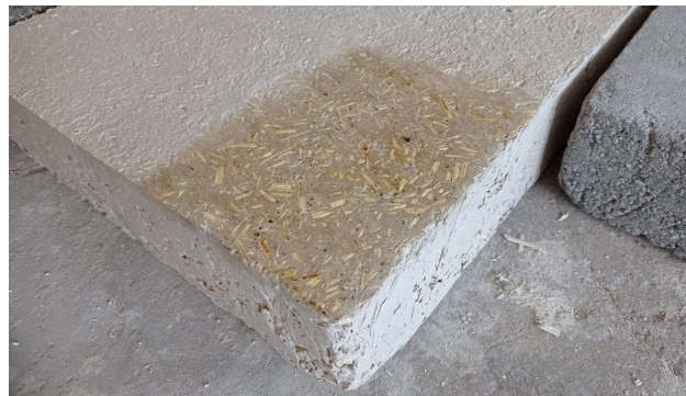
Fig. 7 – HCLS-M sample finished with sand paper and applied a water base stain protection.
