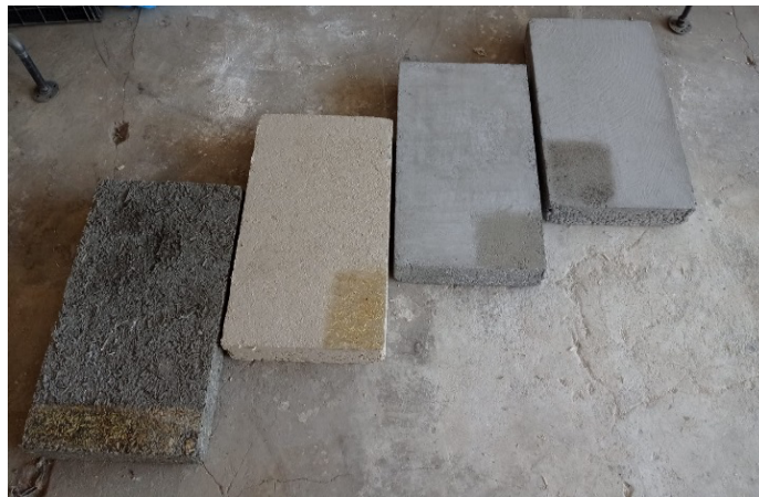
Fig. 3 – Casted samples for different recipe of levelling screed. From left to right: HCLS, HCLS-M, PLS, ECLS.
