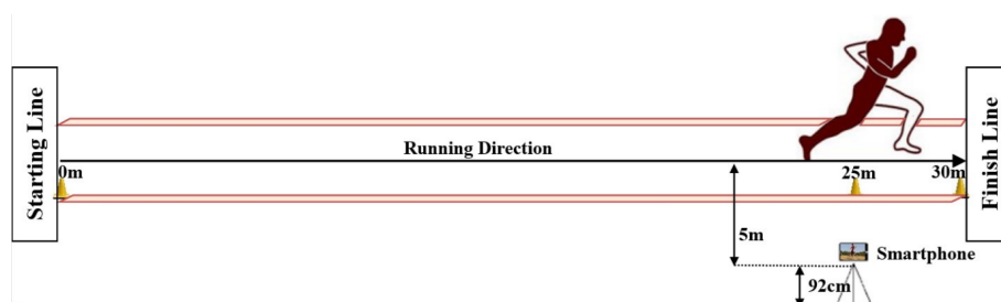
Figure 1. Schematic representation of the experimental setup, providing details of the runway layout and camera positions for capturing the running trials
