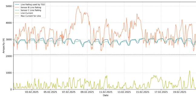
Figure 5: Comparison of the calculated Ampacity for Sensor B (orange), Sensor C (green), current line rating used by APG (blue), max current of the line/static line rating 2080 A (red)
