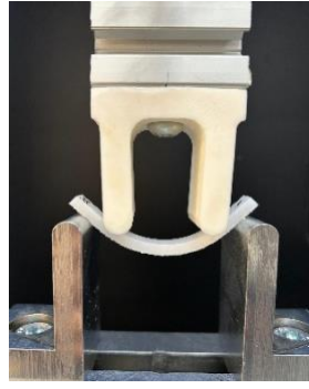
Figure 3: The bending device mounted on Galdabini Quasar 25 testing machine.
