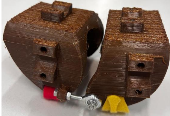
Figure 11 3D printed patient-specific exoskeleton assembled components
