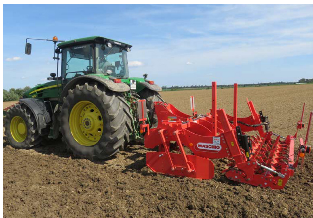
Fig. 1 Machine-tractor aggregate consisting of tractor John Deere 8R280 and subsoiler for soil loosening Maschio-Gaspardo, model Artiglio 300/7 Source: Agronika, 2025
