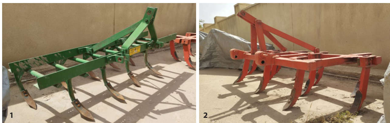
Fig. 1 Two types of chisel plough shank during ploughing 1 – flexible type; 2 – rigid type
