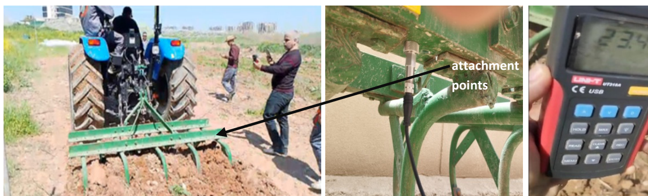
Fig. 2 The device attached to the plough and reading the vibrations during ploughing
