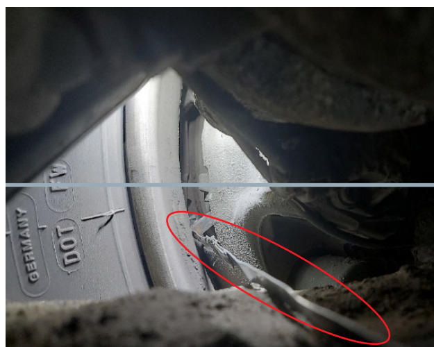
Fig. 2 Measuring the thickness of the brake pads
