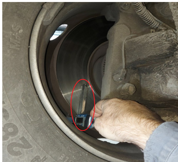
Fig. 1 Measuring brake disc thickness using a digital micrometer
