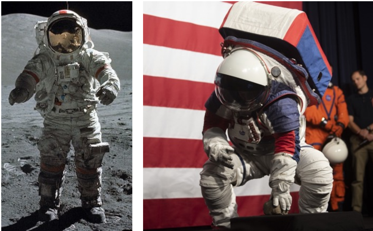
Figure 8. Left: Suit of one Apollo crewmember covered with lunar dust from the waist down. Right: Prototype of the Artemis extra-vehicular activity mobility unit. Image credit NASA.
