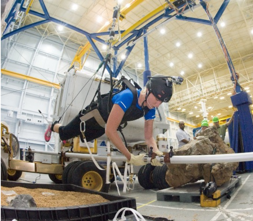
Figure 7. The NASA Active Response Gravity Offload System (ARGOS) simulates reduced gravity by applying a consistent force offload using an overhead hoist system and horizontal movement via a rail and trolley setup. Image credit NASA.
