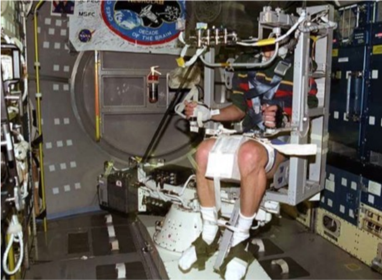
Figure 9. Short-arm human centrifuge utilized on board Spacelab in 1998 to study the effects of artificial gravity on the vestibular system of astronauts. Image credit NASA.
