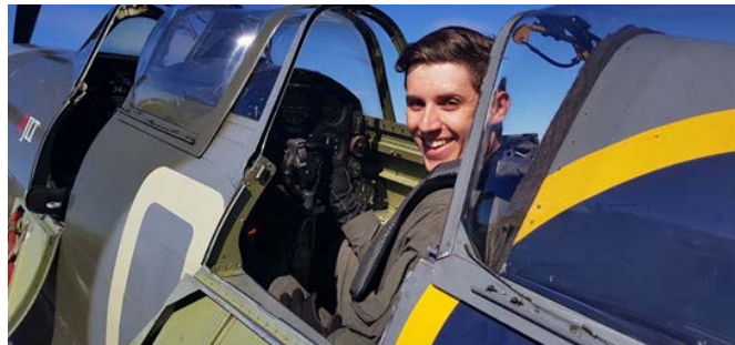
Image 9. Spitfire Mk IX cockpit. The author is seen here in the rear cockpit. Note that the blind flying panel sits just below DEL and within the 30 degree arc for optimal viewing. (1)
