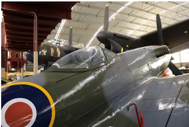
Image 11. Bubble canopy feature on the F.22 Spitfire, showing rear armour plating and fantastic all-round visibility. (1,7)
