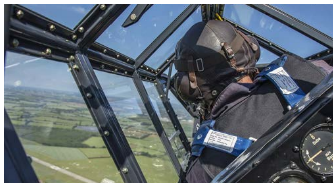
Image 10. Rear cockpit in Ha-112 Buchon. The instrument panel sits well below the DEL and 30 degree viewing arc. Note the tight canopy clearance. (Image adapted from Ultimate Warbirds) (6)
