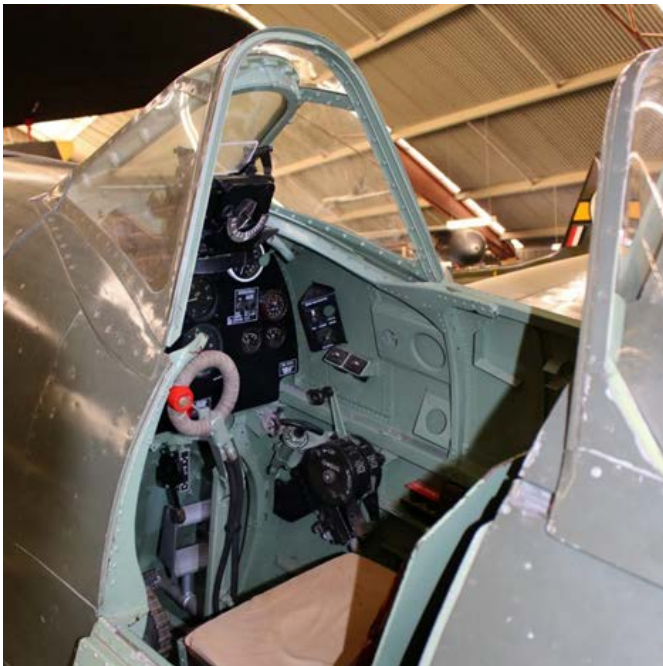
Image 1. Spitfire F.22 Cockpit entry. Car door, seat, spade grip, landing gear actuator, gyroscopic gunsight and part of instrument panel are seen here. (1, 7)
