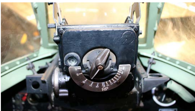
Image 8. Gyroscopic gunsight of the Spitfire F. 22. This image was taken at the DEL. (1, 7)
