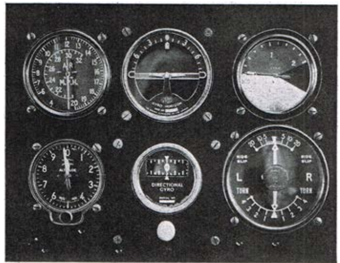
How the instruments are arranged in the new panel. From left to right they can be seen as: (top) Airspeed indicator, Artificial Horizon and rate-of-climb indicator; (bottom) sensitive altimeter, Directional Gyro and turn and bank indicator. This particular rate-of-climb indicator is shortly to be replaced by an improved type. (R.A.F. Official: Crown Copyright Reserved.)
