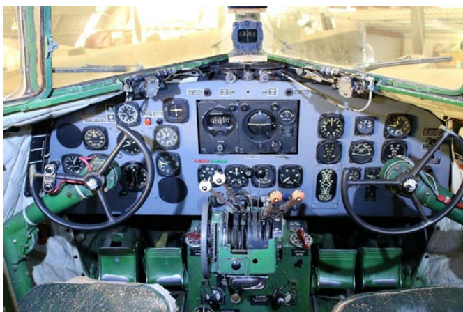
Image 5. C-47 Dakota cockpit. Note the central instrument cluster for blind flying. There is also insulation throughout the cockpit for pilot comfort. (1,7)
