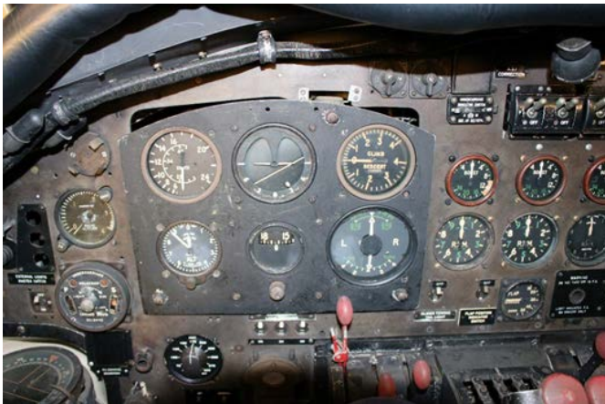
Image 7. Lancaster B2 instrument panel. Despite the vastly different role and configuration of the Lancaster bomber, it features a near identical Blind Flying Panel. (1, 7)
