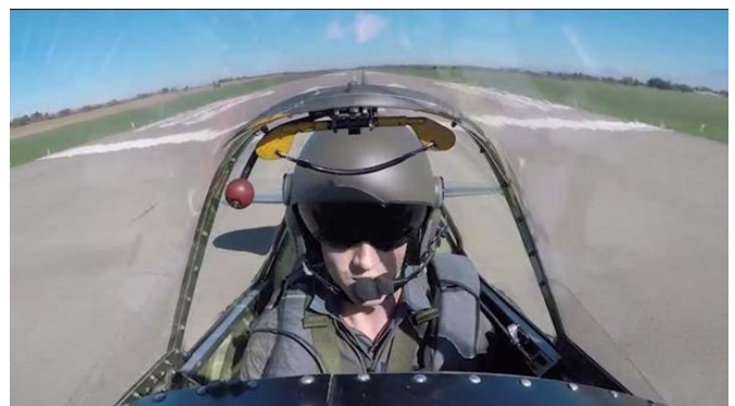
Image 13. Spitfire Mk IX rear canopy. Excellent rearward visibility is seen here (even with the high rear fuselage), as well as the later model ball-toggle canopy release. (Image adapted from Ultimate Warbirds) (1,6)
