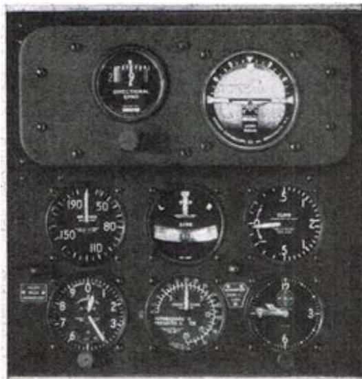
A typical American array of a few years ago, used on the Boeing 247s. Above is the Sperry-free gyro panel, while below, from left to right, can be seen (top row) an A.S.I., a turn and bank indicator, and a rate-of-climb indicator, and (bottom row) a sensitive altimeter, a boost gauge, and a clock.
