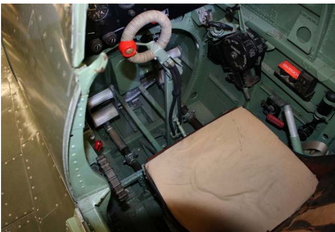
Image 2. Spitfire F. 22 cockpit. Seat (with height adjustment lever and harness), spade grip, rudder pedals, landing gear actuator, trim wheel and part of instrument panel seen. A pillow is provided for comfort in place of the Seat-Type Parachute. (1, 7)
