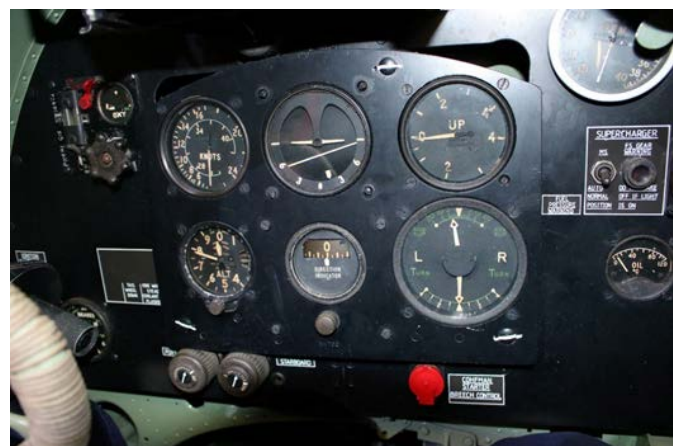
Image 6. Spitfire F.22 instrument panel, featuring the Blind Flying Panel. Note the ancillary engine gauges to the right, as well as oxygen system controls to the left. (1,7)
