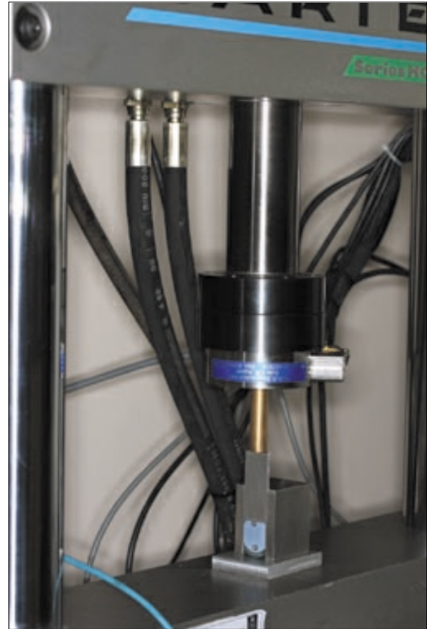
Figure 2. Jig mounted in Dartec Series HC10 for cyclic fatigue loading, showing two opposing brackets in position.
