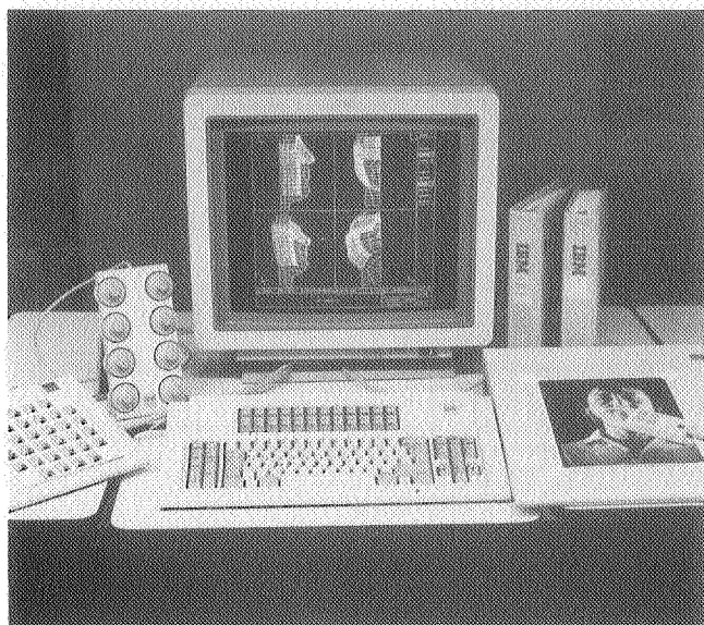
Figure 4. IBM™ Work Station (a) digitising pad (b) high resolution screen (c) image control unit
