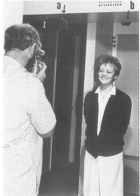
Figure 4. Camera - subject relationship. Note : Main flash unit (arrow a), Background flash unit (arrow b), Background (arrow c)
