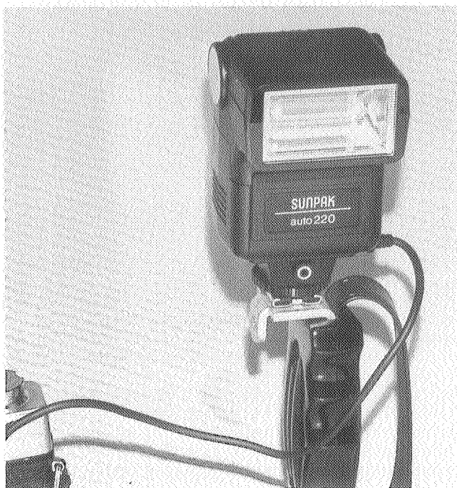
Figure 3. Flash unit mount. Note : Synchronisation cord
